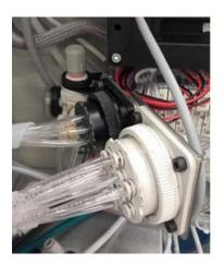
Connect the flying pneumatic connectors, located on the miniapplicator, with the panel on the back of equipment. Make sure that the locking rings are inserted and tightened.
