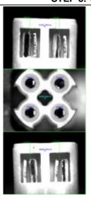
At the same time the wire is locked, the video cameras photograph and verify the quality of the process occurred in station 6. In sequence, they evaluate the left side, from the top, and the right side.
