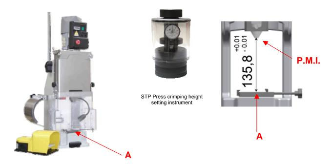
Press crimping height setting is very important for correct operation. Clean the baseplate surfaces "A", guaranteeing a good support surface between the base of the press and that of the mini-applicator. Use the corresponding STP Crimping height instrument to verify the correct working height which must be BDC 135.8mm (±0.01mm).
