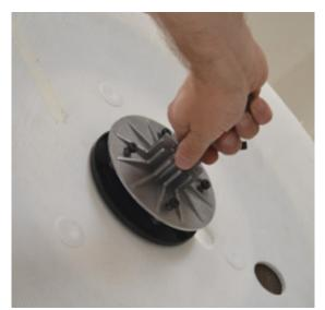
Remove the fixing flange and replace the reel.
