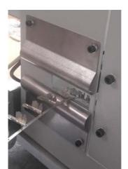
Insert the strip inside the machine casing, having it pass from the slot on the left side of the equipment.
