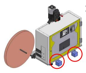
Close the fixed casing back up and activate the two-hand control for reset.
