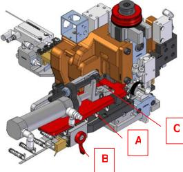
Insert the terminal to be crimped in the guide **A** after having freed the clutch by means of the eccentric part **B**. Push the strip terminal until it engages with the pawl **C** and close the clutch.
