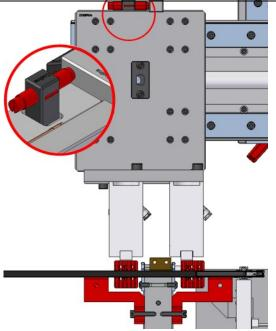
Unscrew the fixing nut and adjust the decelerator. The top clamp unit must be centred with the wire support on the bottom unit. Tighten or loosen to find the correct position. Re-screw the lock nut again on the decelerator.
