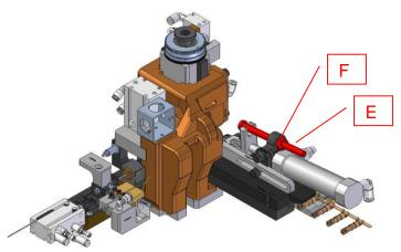
The terminal arrival position is defined by the cylinder stroke. Loosen the lock nut F and regulate the adjustment screw E. Once the correct position has been found, re-tighten the lock nut F. Repeat the operation until the desired adjustment has been set.
