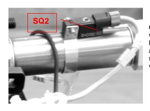
Once the pitch has been adjusted, proceed with the sensor with detects cylinder position.
