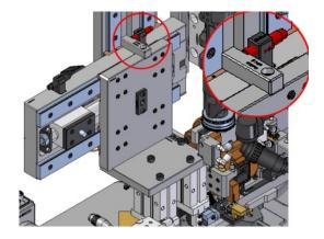
Using the decelerator, mechanically adjust the position of the top manipulator so as to obtain the minimum measurement of insulator insertion in the OUTER/BODY contact.
