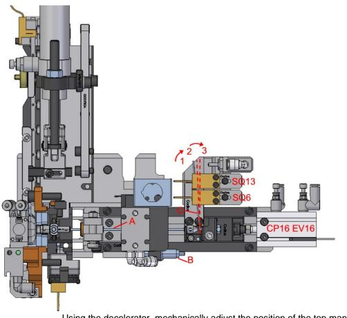
Using the decelerator, mechanically adjust the position of the top manipulator so as to obtain the minimum measurement of insulator insertion in the OUTER/BODY contact. The insertion positions to maintain are 2.35 for the Female contact and 5.45 for the Male contact.
