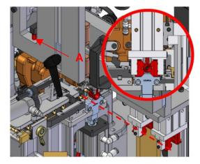
Clamp unit alignment with respect to the terminal is decided by decelerator "A".
