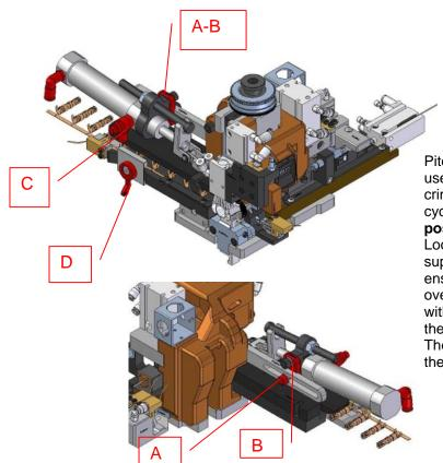
Pitch P adjustment on the Magnum applicator is used to engage the terminal and move it to crimping position during each complete operating cycle. The terminal must be set in the crimping position with clutch D in the operating phase. Loosen the locking screw A and move the support B until adjustment has been made. To ensure correct adjustment, move the pawl slightly over the anchoring point (normally corresponds with the hole or slot present on the strip). Tighten the locking screw A.
