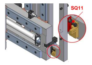
Unscrew the fixing screw on the sensor SQ11 level and move the sensor lever upward, bringing it outside the sensor reading field.
