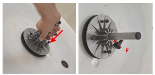
Re-insert the flange, slightly press down, pushing the flange toward the reel. Secure the position, tightening the locking handle F.
