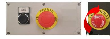
To restore the emergency, release the button, turning it in the clockwise direction until you hear a release "click."
