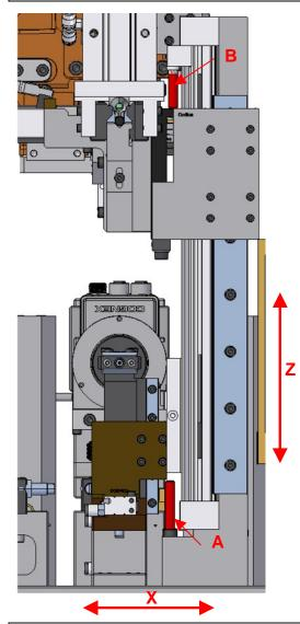
The wire support unit is adjusted by two dowels.
