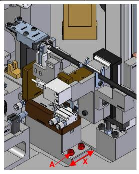
Adjust axiality in X of the insulator reference with respect to the wire support unit, unscrewing the screws "A". Re-tighten all screws once adjustment has been made.
