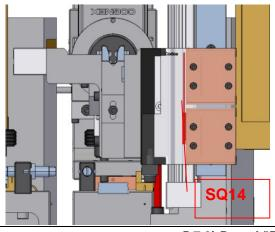
Move the wire support unit to an aligned position with the insulator reference. Unscrew the screw on sensor SQ14 and move it upward, slowly bring the sensor down, searching for cylinder position recognition. The LED will switch on when the position has been reached. Fix the sensor and verify a couple times that adjustment has been performed correctly, activating solenoid valve EV10.
