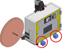
STEP 6. Cycle end At the end of the cycle, the mobile guard opens automatically, the wire is freed and the operator can remove it.
