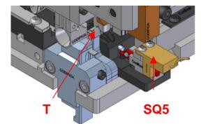
Presence sensor SQ5 is activated under the condition that terminal T is positioned and locked correctly in its housing.
