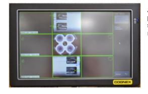
At the same time the wire is locked, the video cameras photograph and verify the quality of the process occurred in station 6. In sequence, they evaluate the left side, from the rear, and the right side.
