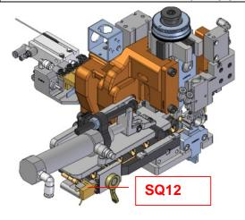
The optical sensor (SQ12) verifies the presence of Outer terminal banding strips. It is always active and does not have any adjustments. When the strip ends, the sensor deactivates the signal, sending an error message to the press. <u>Replace</u> the finished reel with a new one.
