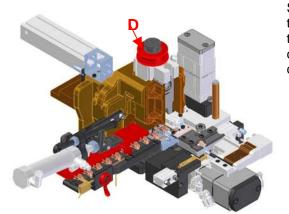
Sample the section of the wire to be used, having arranged the adjusting ring "Copper D" as indicated by the values on the plate located on the applicator body. If the detected crimping height does not correspond with said references, check:
