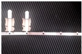
Before inserting the terminal strip in the mini-applicator, cut the first 4 or 5 terminals as shown in the figure.
