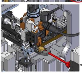
Fasten the base of the applicator to the base of the press, screwing the rod into the base.
