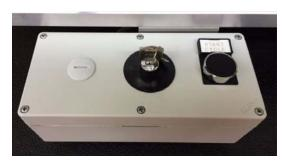
Re-lock the system using the key, moving to the LOCK position.
