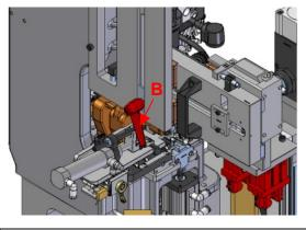
Loosen the fixing handle "B" and move the unit upward. Loosen the fixing nut on the decelerator "A" and adjust the dowel, loosening it (clamps raise) or tightening it (clamps lower). Lower the unit again, bringing it to the reference position on the decelerator and making sure that it has reached the desired position. Secure the nut on the decelerator "A".
