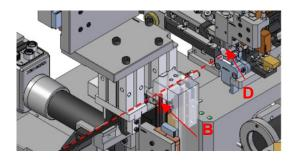
Unscrew the fixing nut on dowel "B", adjust the dowel so that the wire support unit is aligned with the terminal and the funnel "D". Re-lock the nut.
