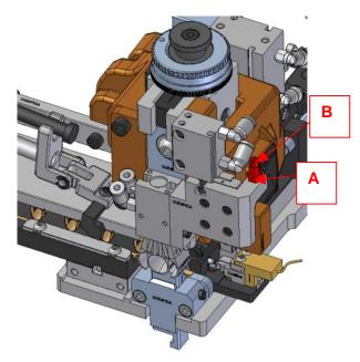
Lock the terminal with the presser, activating the solenoid valve EV15. Cut the strip EV5 and lower the funnel with solenoid valve EV14.
