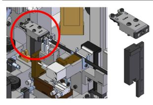
Replace the block and connect the relative connector. Unscrew the fixing screws, replace the block, connect the connector and re-tighten the screws.
