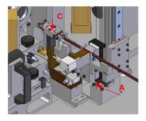
Unscrew the fixing nut on dowel "A", adjust the dowel so that the wire support unit is aligned with the insulator reference "C". Re-lock the nut.
