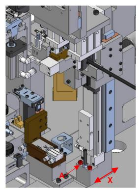
Activate EV10, moving the wire support unit to the wire release position (upward).
