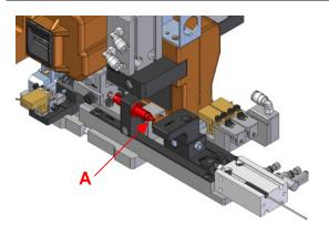
Correct placement of the insulator in the terminal is verified by two sensors SQ6 and SQ13, which are activated by their relative sensor lever.
