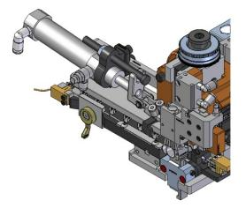
Unscrew the floating blade cover screws, remove the cover and the floating blade and replace the anvils. Re-insert the floating blade cover and the blade, re-tighten screws.
