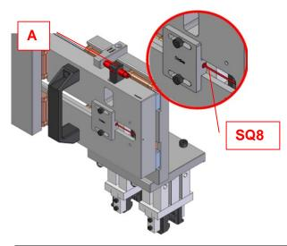
The sensor SQ8 detects clamp position, giving consent to the wire support unit to move upward.
