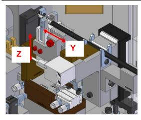
After having inserted the wire in the insulator reference, the pneumatic clamp will being operation, locking the insulator and ensuring its position during verification by the video cameras.
