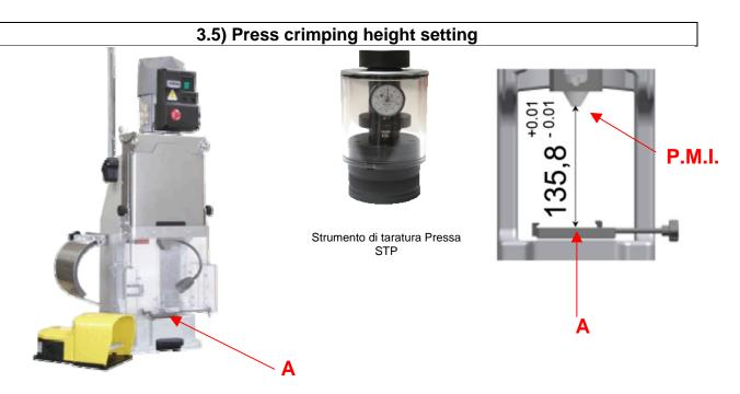
Press crimping height setting is very important for correct operation. Clean the baseplate surfaces "**A**", guaranteeing a good support surface between the base of the press and that of the mini-applicator. Use the corresponding STP Crimping height instrument to verify the correct working height which must be BDC 135.8mm ( $\pm 0.01$ mm).
