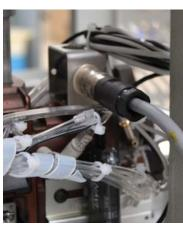
Connect the flying electric connector located on the machine with the panel connector positioned on the miniapplicator. Make sure that the locking ring is inserted and tightened.
