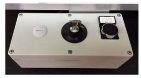
Use the key to unlock, moving to the UNLOCK position.
