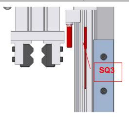
Move the wire support unit to an aligned position with the terminal and funnel, activating solenoid valve EV10. Unscrew the screw on sensor SQ3 and move it downward, slowly bring the sensor up, searching for cylinder position recognition. The LED will switch on when the position has been reached.
