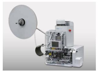
▲ Komax bt 712 with programmable stripping device
