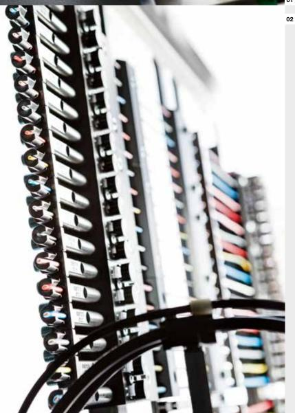
The bundler sorts and binds the batches in a single process step. 02 Up to 36 different cables from the entire cross section range are available in the wire selector.
