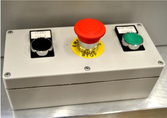
**If you need to stop the machine at any time during the cycle, press the emergency button. The emergency button cuts off power to equipment and discharges the pneumatic system.**
