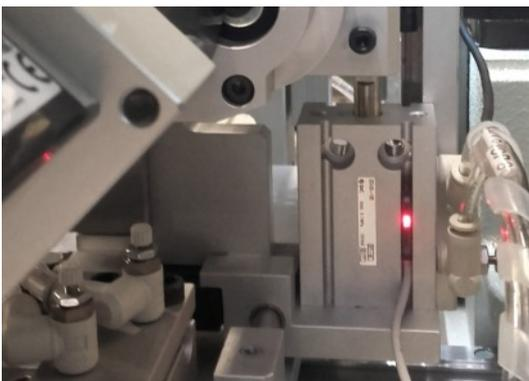
The sensor gives consent to the control unit when the table is in the raised position. To adjust it, make sure that the table is positioned upward, insert the sensor until the red LED lights up and fasten the screw.
