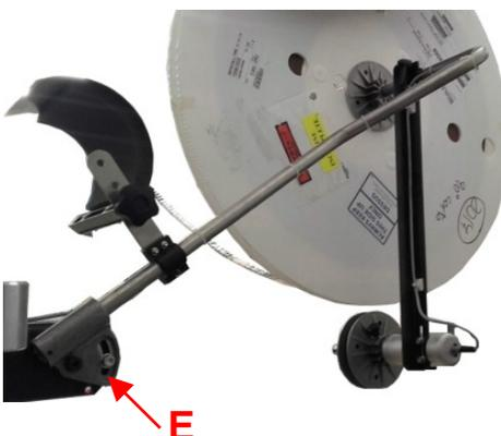
The terminal reel to be processed with the left mini-applicator is supported by the dereeler installed on the left side of the equipment.
