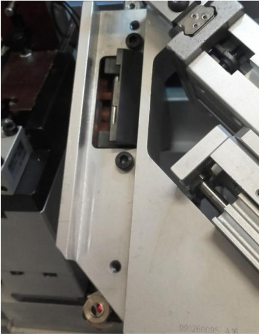
Close the cable locking clamp, pushing it to the left.
