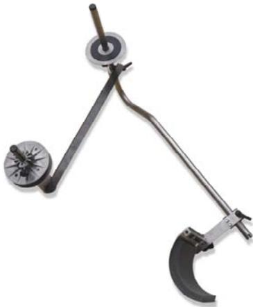
The left press dereeler will have to be assembled as in the figure, with the curved plate **A** and the paper winder motor **B** turned to the left.
