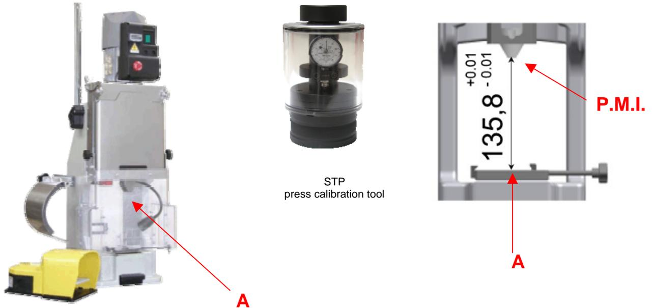
Press calibration is very important for correct operation. Clean clamping surfaces “A,” ensuring a suitable support surface between the base of the press and that of the mini-applicator. Use the STP Calibration Tool to verify the correct working height, which should be BDC 135.8mm ( $\pm 0.01$ mm).
