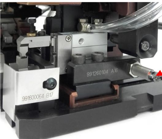
Adjust the decelerator to adjust the clamp unit with respect to the y axis.
