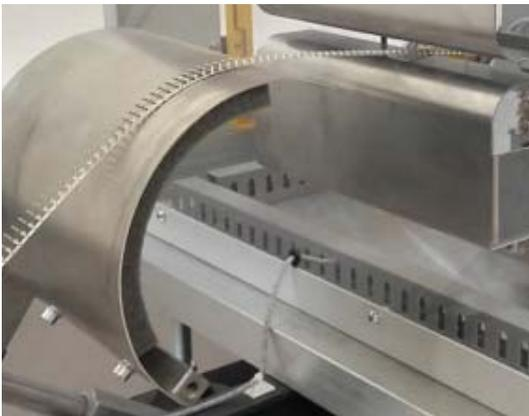
Slide the terminals over the curved plate on the left side of the press and insert it in the slot.
