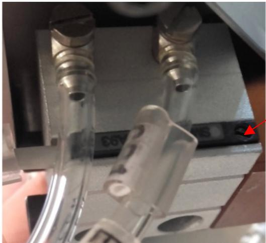
Insert the sensor in the cylinder housing and push it slightly until the red LED switches on. Secure the sensor by tightening the screw.
