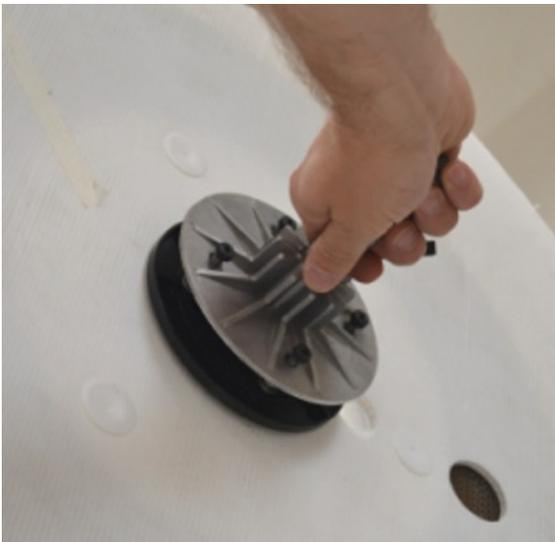
Insert the fixing flange, bringing it to end stop on the reel surface.
