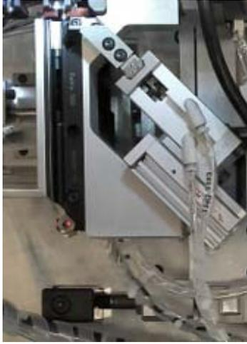
The HSD cable is composed of 4 internal cables which need to be crimped individually. Cables are preventively moved apart to ensure this process.
