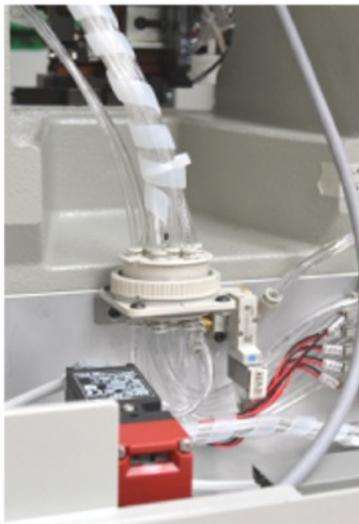
Connect the flying pneumatic connectors, located on the mini-applicator, with the panel pneumatic connectors on the back of equipment. Make sure that the locking washers are inserted and tightened.
