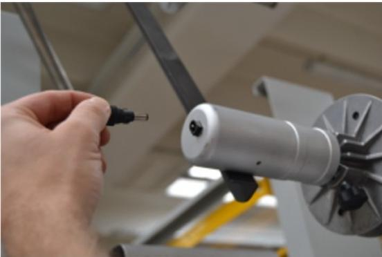
Connect the power cables on the machine to both paper winder motors.
