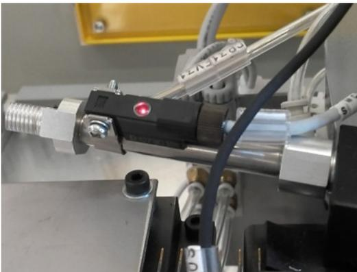
The sensor (SQ32 left mini-applicator and SQ33 right mini-applicator) on the centring device cylinder is adjusted by detecting the cylinder stand-by position. Insert the sensor and secure it as soon as the red LED lights up.
