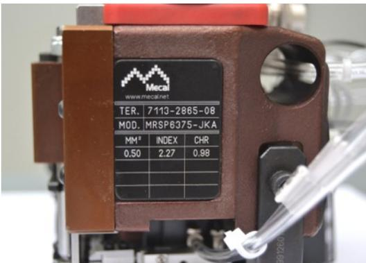
Adjust the ring nut according to the "INDEX" value contained on the identification plate and corresponding to the cross section of the cable to be processed. INDEX represents the operating position of the centesimal ring nut. In the example photo, the value for the only cross section present is 0.50 mm<sup>2</sup> is equal to 2.27 mm.
