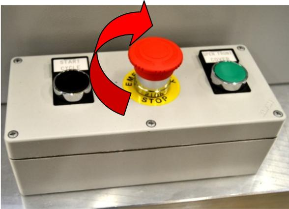
To restore the emergency, release the button, turning it in the clockwise direction until you hear a release "click."
