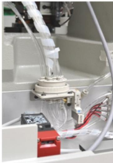
Connect the flying pneumatic connectors, located on the mini-applicator, with the panel pneumatic connectors on the back of equipment. Make sure that the locking washers are inserted and tightened.
