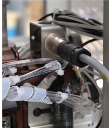
Connect the electrical flying connector on the machine with the panel connector located on the mini-applicator. Make sure that the locking washer is inserted and tightened.
