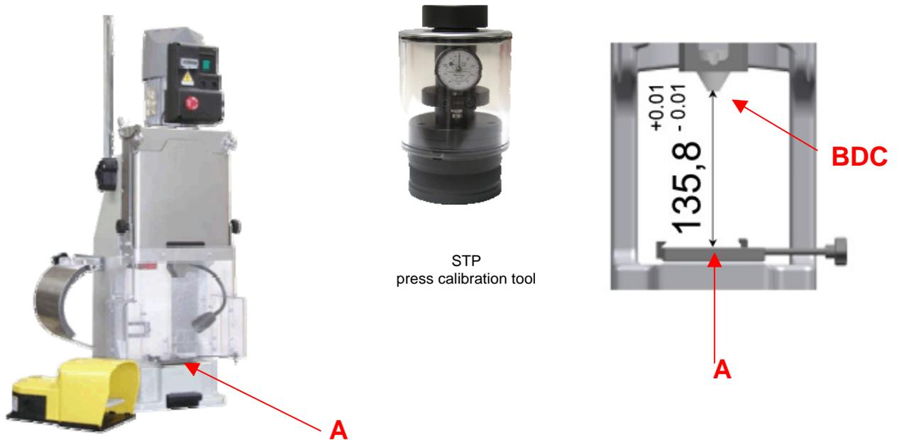
Correct press operation is guaranteed by its relative calibration. Clean clamping surfaces "A," ensuring a suitable support surface between the base of the press and that of the mini-applicator. Use the STP Calibration Tool to verify the correct working height, which should be BDC 135.8mm ( $\pm 0.01$ mm).
