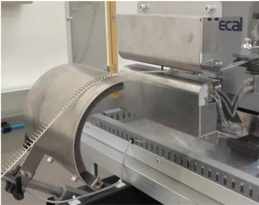
Insert the strip inside the machine casing as shown in the figure.
