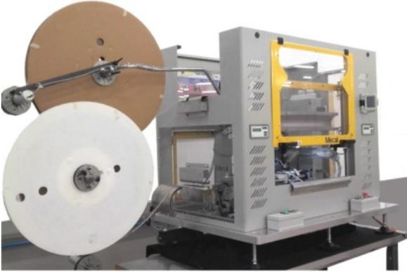
Insert the terminal reel on the overhanging part of the dereeler rod.
