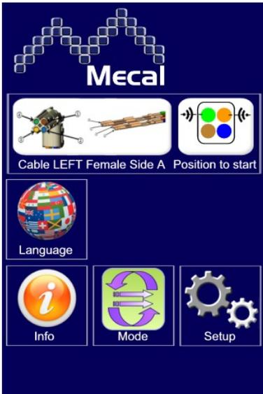
The Home Screen is divided into two parts: the upper one, NOT selectable, specifies to the operator how cable colours that he has decided to crimp should be positioned.
