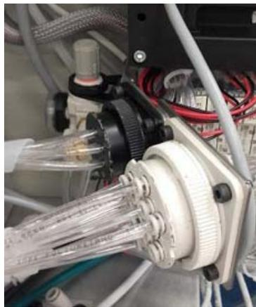
Connect the flying pneumatic connectors, located on the mini-applicator, with the panel on the back of equipment. Make sure that the locking rings are inserted and tightened.
