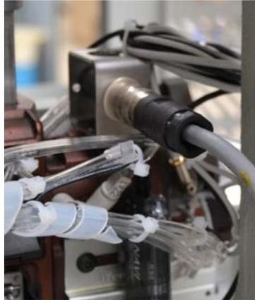
Connect the flying electric connector located on the machine with the panel connector positioned on the mini-applicator. Make sure that the locking ring is inserted and tightened.
