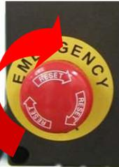
To restore the emergency, release the button, turning it in the clockwise direction until you hear a release "click."
