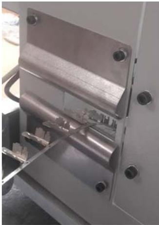
Insert the strip inside the machine casing, having it pass from the slot on the left side of the equipment.
