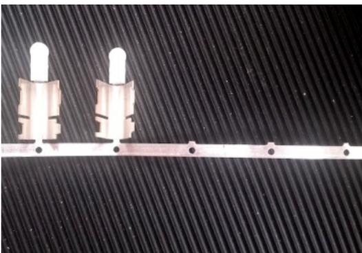
Before inserting the terminal strip in the mini-applicator, cut the first 4 or 5 terminals as shown in the figure.
