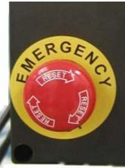
If you need to stop the machine at any time during the cycle, press one of the two emergency buttons.
