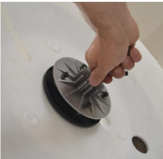
Remove the fixing flange and replace the reel.
