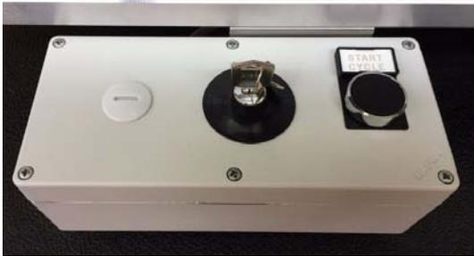
Re-lock the system using the key, moving to the LOCK position.
