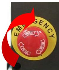
To restore the emergency, release the button, turning it in the clockwise direction until you hear a release "click."
