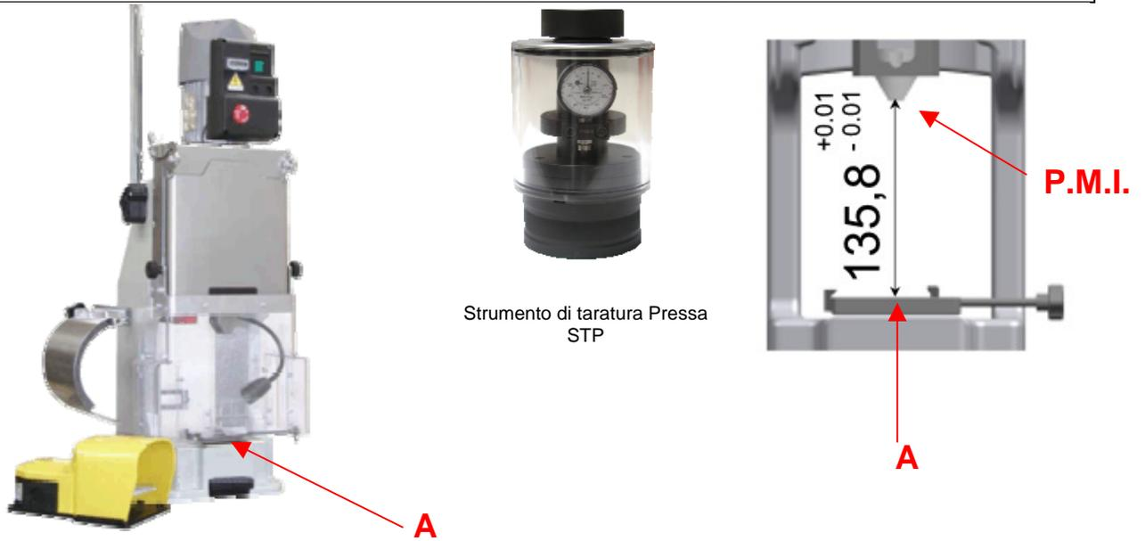
Press crimping height setting is very important for correct operation. Clean the baseplate surfaces “A”, guaranteeing a good support surface between the base of the press and that of the mini-applicator. Use the corresponding STP Crimping height instrument to verify the correct working height which must be BDC 135.8mm ( $\pm 0.01$ mm).
